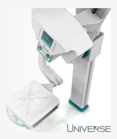
The Universe™ includes various safety features to prevent patient risk. The collision prevention system uses photoelectric sensors to slow down or stop the U-Arm movement if any obstacle is detected while in operation. Collision sensors on both the U-Arm stand and the detector react to any unexpected shock.
